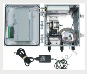
The Backup Battery Kit includes a -48V DC power supply, which converts 115V AC power at the dryer to -48V DC (required for the uM260). It also includes a backup battery, which temporarily powers the monitor if disruption of AC power occurs. Included with the battery and power supply are the necessary power cables, plus an AC alarm pair and a power pair for the uM260.
