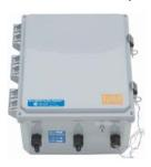
The Remote Dryer Monitoring Kit is a self-contained, encased monitoring assembly designed for installation at a remote air dryer location. It can be installed either inside the dryer cabinet or placed on the pole below it. The kit is comprised of a rugged plastic cast containing the modem version of the uM260 Micro Monitor (Part No. 9800-6260M), our uM260 Backup Battery Kit
