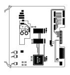
This version of the 289H Utility Card makes it possible to transmit a pseudo-data tone or a selected tone frequency (locator tone) on the monitoring device pairs wired to the 289H monitor. Works in either capacity with all dedicated relay cards manufactured after December, 1998 (Rev. C and above). Locator tone capability only is available for subscriber cards.
