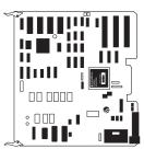
The controller card performs most of the tasks that direct the operation of the 289H and its interaction with the PressureMAP™ software. It is available here as a replacement card.
