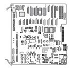
The controller card performs most of the tasks that direct the operation of the 289H and its interaction with the PressureMAP software. The latest version of the card includes an onboard local area network (LAN) adapter and over-voltage protection for the 289H's measurement circuit.
