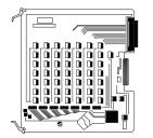
The Sparton Dedicated Replacement Card (SPDR) streamlines the process of cutting over from a Sparton monitor to the 289H or 289H-M LSS. SPDR Cards can be configured to accept the Sparton dedicated block's A, B or C cables. No additional adapters or connectors are required.
