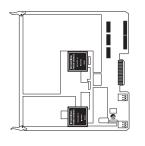
The utility card contains a 48 volt DC power supply, a microprocessor which contains the I/O circuitry for the 289H chassis, a power switch, and an alarm enable/disable switch. This card is supplied with the 289H and 289H-M monitors. It is also required when an expansion chassis is used with the 289H LSS. It provides the interface to
