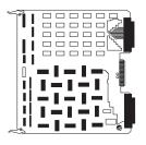
The subscriber relay card is the Loop Surveillance System's internal termination point for transducers installed on subscriber device circuits. Because of its architecture and relay configuration, it is also possible to use dedicated circuits with this card. The card accommodates a maximum of 25 devices.
