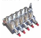
This version of the Flow Bank is supplied with five nickel-plated brass, 1/4" NPT to 3/8" tubing connector fittings. Internal Flow Finders are standard 0-9.5 SCFH. The 3/8" brass fittings are the standard in most U.S. Telcos.
