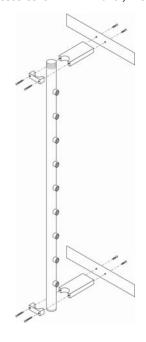
This 9-Port Manifold Kit is supplied as a retrofit for existing equipment racks that use weak Schedule 40 (white) PVC rack manifolds. It is supplied with a stainless steel manifold, required connectors, plugs, bushing, etc. Manifold length is 72 in (183 cm); internal diameter is 2 in (5.08 cm).
