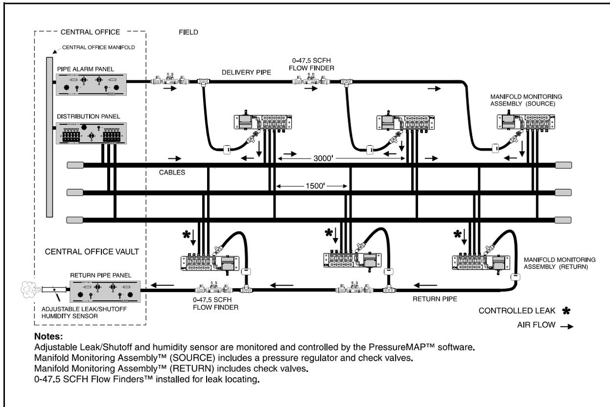
FIGURE 1: THE POSITIVE AIR FLOW SYSTEM
