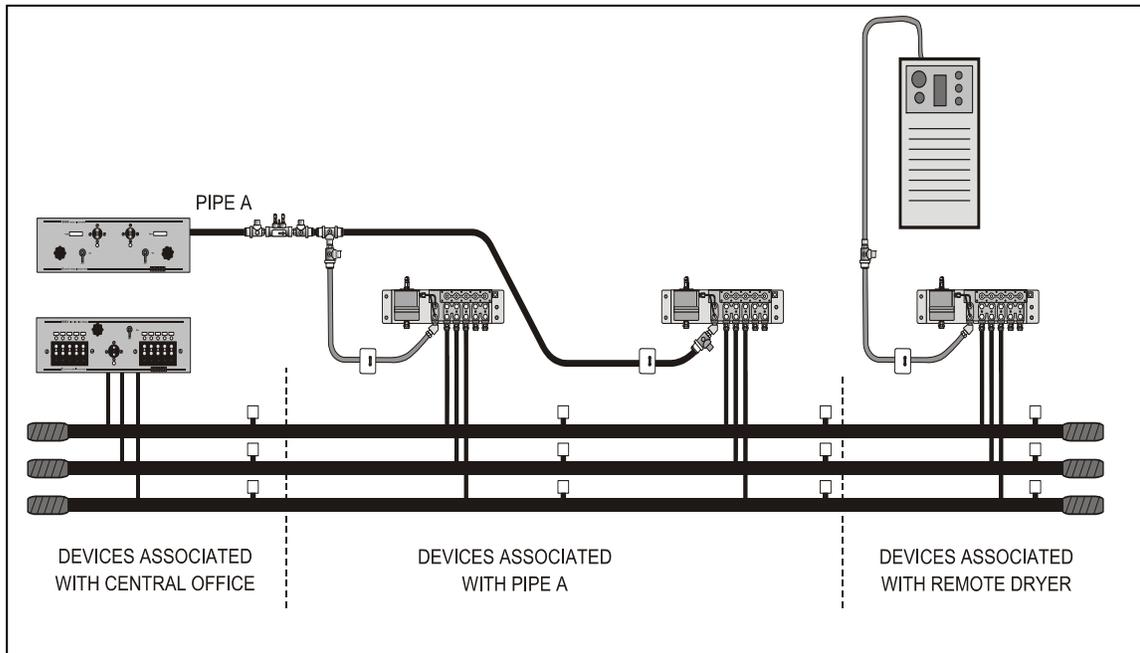
FIGURE 6-1: DEVICES ON OFFICE SIDE OF A REMOTE DRYER
